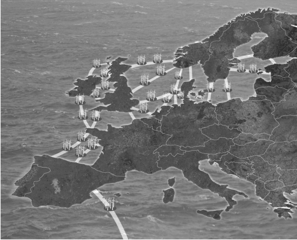
Figure 8.3 Concept map of the proposed European DC supergrid. (Reproduced with permission of Airtricity)
