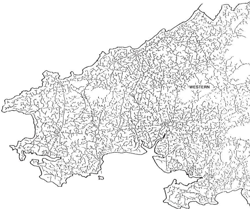
Figure 5.7 11 kV in South Wales on the same scale
